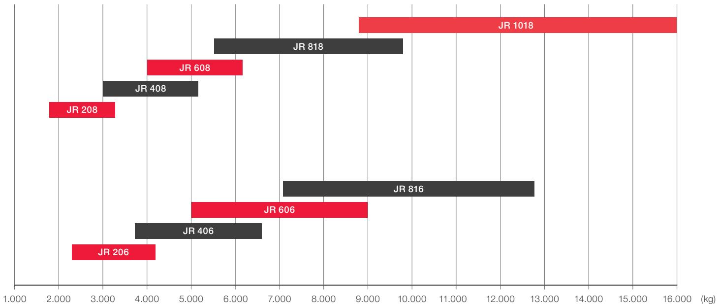
Construction weight when using one exciter.
